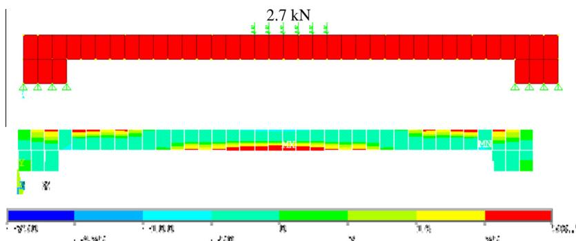
Fig. 9 Numerical nonlinear analysis results for beam B.
