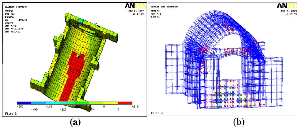
Fig. 16 Nonlinear analysis results; (a) stresses  $S_x$  and (b) crack pattern.
