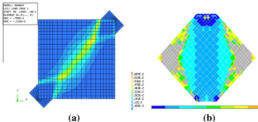
**Fig. 11** Finite element analysis stresses; (a) stresses in published results [20] and (b) stresses obtained in present work.
