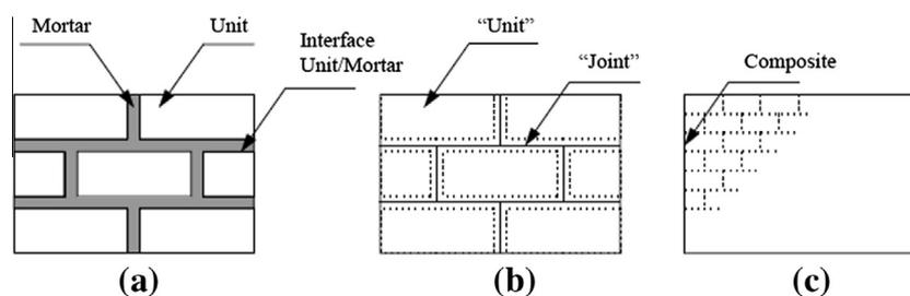
**Fig. 1** Modeling strategies for masonry structures: (a) detailed micro-modeling; (b) simplified micro-modeling and (c) macro-modeling [5].
