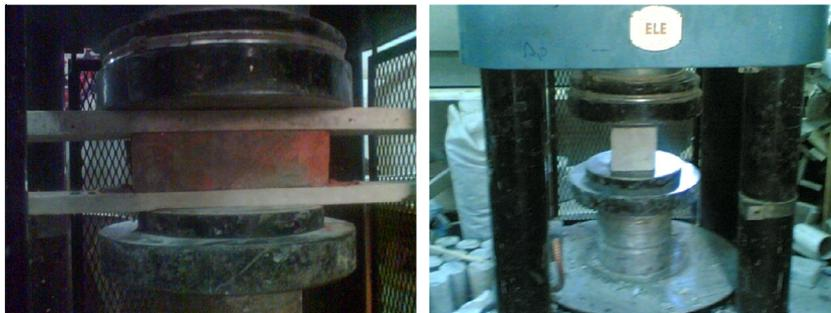
Fig. 5 Compression test for masonry units and mortar cubes.
