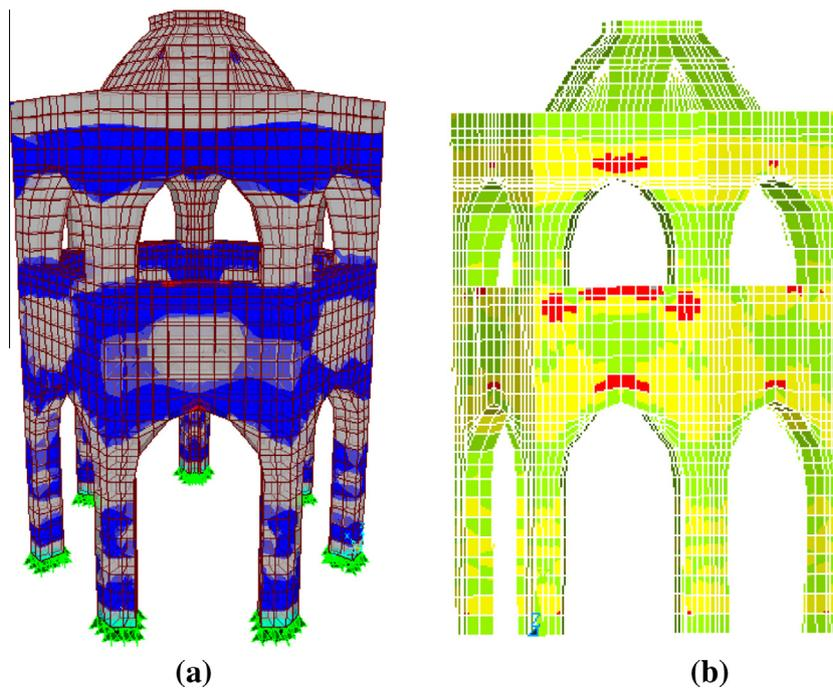
Fig. 17 Finite element analysis results; (a) SAP results and (b) ANSYS results.
