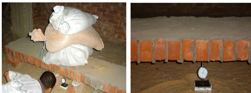
Fig. 8 Loading and instrumentation for beam B.
