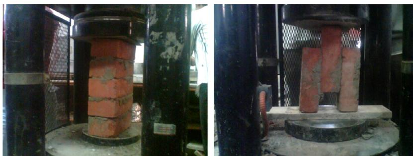
Fig. 6 Masonry prism test and shear bond test.
