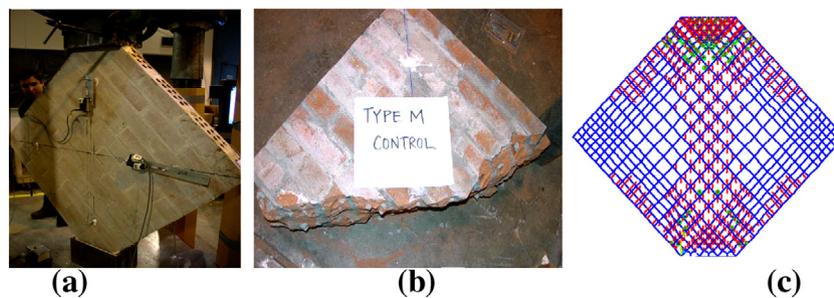
**Fig. 10** Experimental and numerical results; (a) tested panel [20], (b) failure of sample [20] and (c) crack pattern of present study obtained by ANSYS model.
