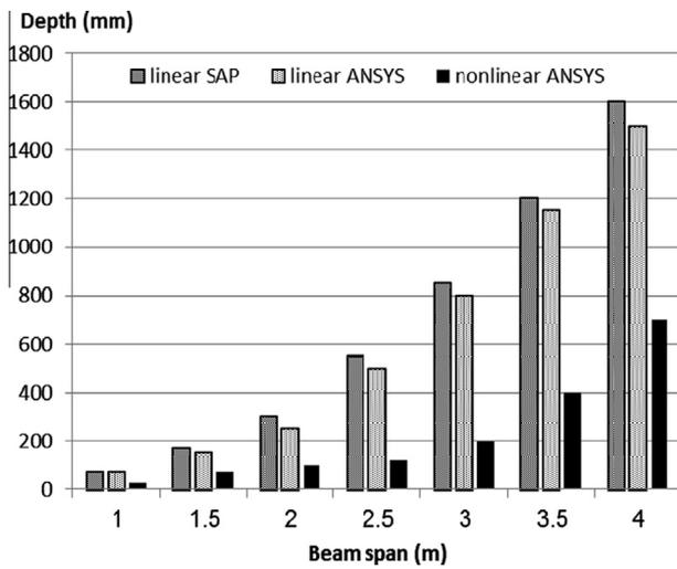
Fig. 4 Comparison between linear and nonlinear results for the studied masonry beams.
